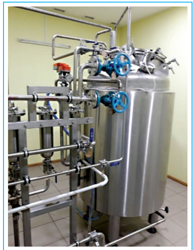
Fermenter for obtaining small batches of the biopreparation based on the B. amyloliquefaciens subsp. plantarum IMB B-7524 strain
