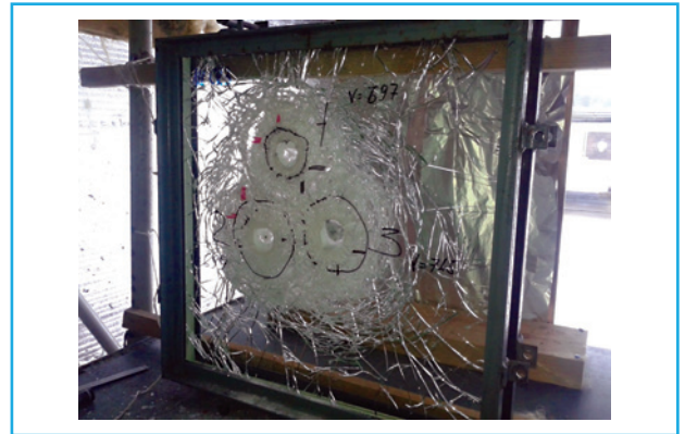
Armored unit for ballistic protection after positive ballistic tests of CK 3 ДСТУ4546:2006 class
