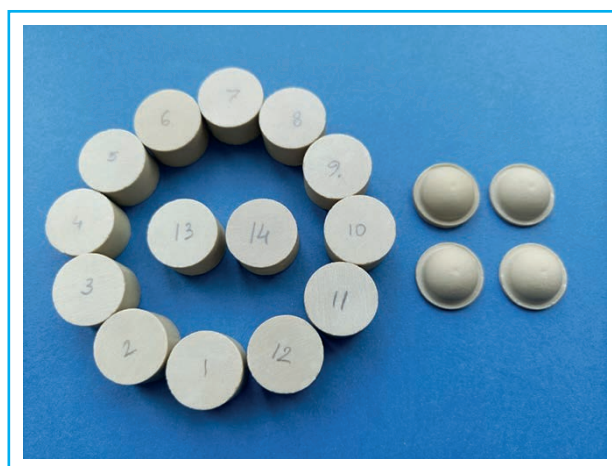
Dielectric resonators for the frequency \sim 5 \text{ GHz} — cylindrical and hemispherical ones
