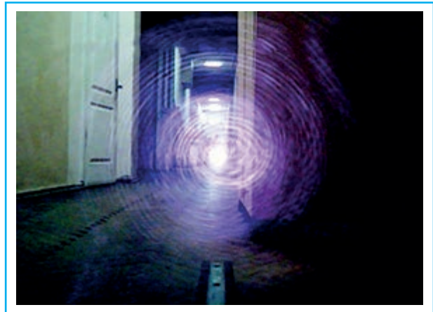
Demonstration of video camera blinding by a laser
