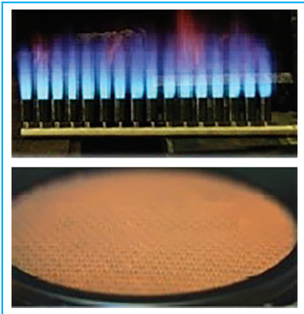
Flare (top) and flameless (bottom) combustion
