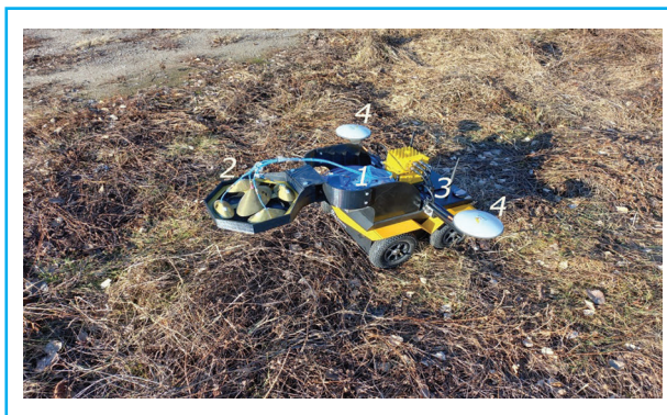
Georadar for detecting explosive objects: 1 – hardware unit; 2 – antenna system; 3 – robotic platform; 4 – GPS antennas
